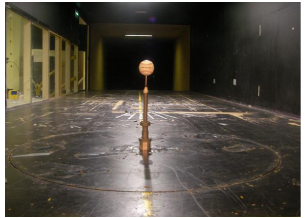
Fig 5. Vertical experimental set up in the wind tunnel
